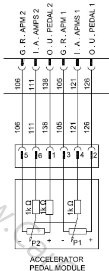
2 The ETC system (Electronic Throttle Control or EGAS)
